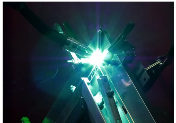
The innovative welding process enables full control of droplet transfer for spatter-free results.
