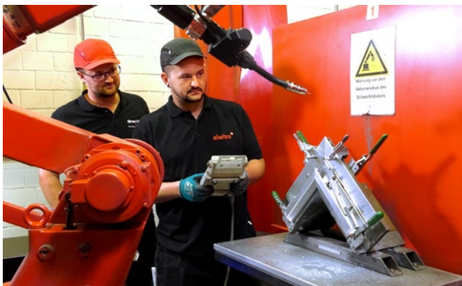
EWM React is a welding process with reversing wire movement which offers maximum control and process reliability for automated MIG/MAG welding.
