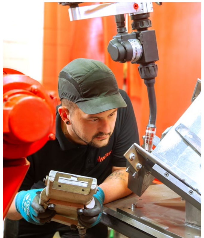
Thanks to the high deposition rate, components can be welded faster with EWM React. At the same time, finishing work is significantly reduced, resulting in a time saving of one minute per workpiece.
